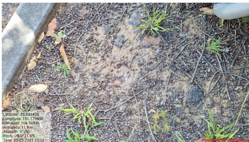
Photograph taken showing the fill evident from the exposed soil in the south western section of the site with inclusions of asphalt and igneous gravel.
